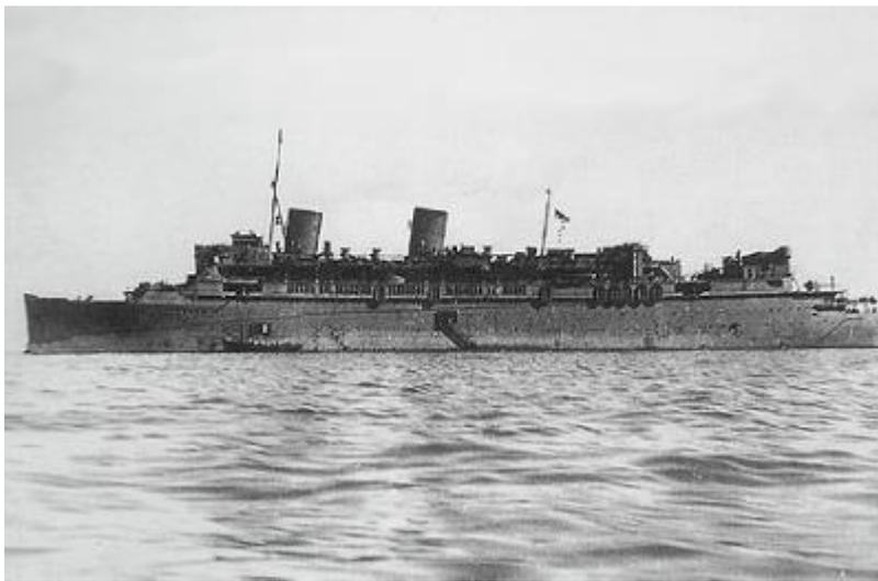
The rear funnel was removed to allow guns to be mounted on the stern.
